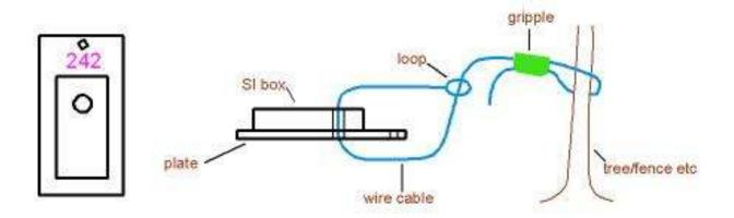
How the wire goes through the Gripple is shown on the next diagram:
