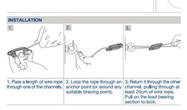
The wire will only move one way through the Gripple, the internal cams prevent the wire from being pulled out. To remove the wire an Adjustment Key is used to release the locking cam in the Gripple. The key is pushed firmly into the small hole below the hole the wire enters and this releases the cam allowing the wire to be pulled out. See below:
